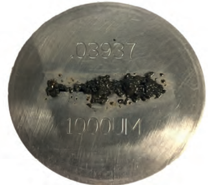
In this example slot test, 20 lb/bbl ENERLOC was added to an unweighted invert emulsion to seal the 1000 micron slot at 500 psi
